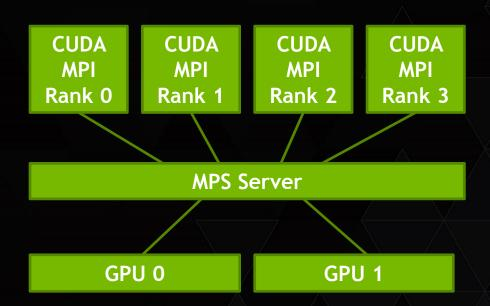
MPS Server efficiently overlaps work from multiple ranks to each GPU
