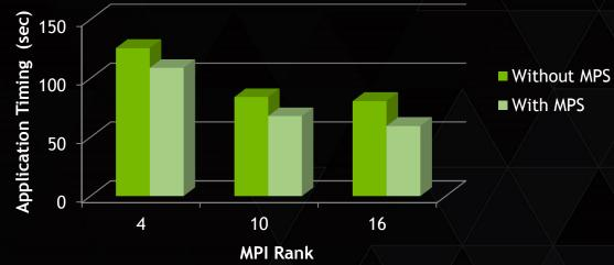
Hyper-Q with multiple MPI ranks on single node sharing same GPU under MPS leads to 1.5X speedup over multiple MPI rank per node without MPS
