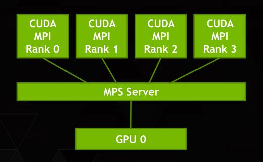
MPS Server efficiently overlaps work from multiple ranks to single GPU
