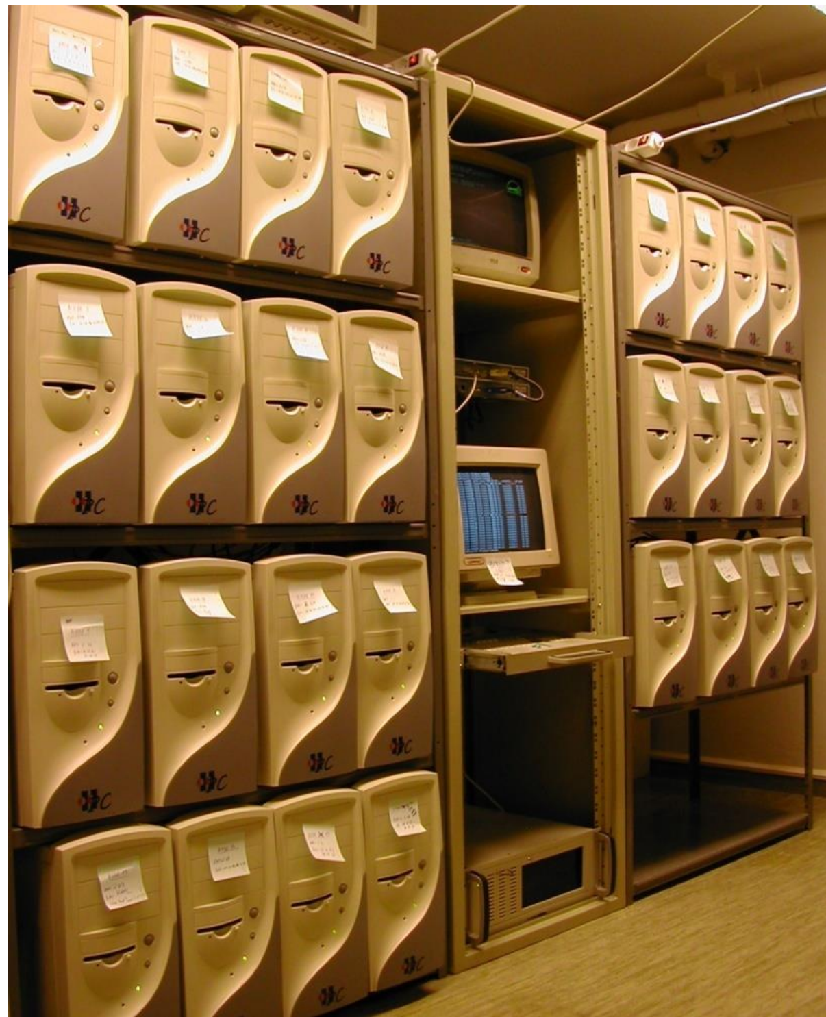
NTNU IDI's 40-node AMD 1.46GHz Cluster w/ 2GB RAM, 40GB disk, Fast Ethernet – ca 2002-2003
