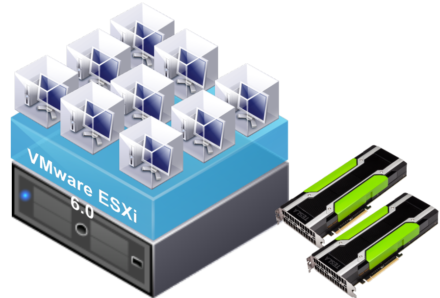
Dell R730 – Intel Haswell CPUs + 2 x NVidia GRID M60 24 cores (2 x 12-core socket) E5-2680 V3 768 GB GB RAM
