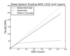
A smaller mini-batch per GPU enables the use of up to 128 GPUs.
