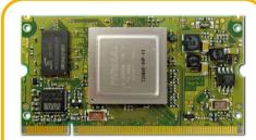
Tegra SoC 1W TDP Cuda GPU SO DIMM
