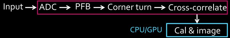
**FX design**: channelise (F), cross-correlate (X) **Hardware**: ASICs, FPGAs, CPUs, GPUs
