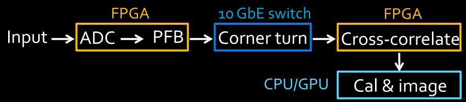
**FX design**: channelise (F), cross-correlate (X) Hardware: ASICs, FPGAs, CPUs, GPUs E.g., LEDA, MWA, PAPER FPGA 10/40 GbE switch GPU Input  $\rightarrow$  ADC  $\rightarrow$  PFB  $\rightarrow$  Corner turn  $\rightarrow$  Cross-correlate Cal & image CPU/GPU
