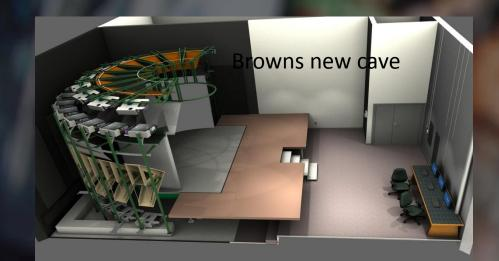
69 1920 1080P 120 hertz projectors Rear Projected Camera Based Tracking
