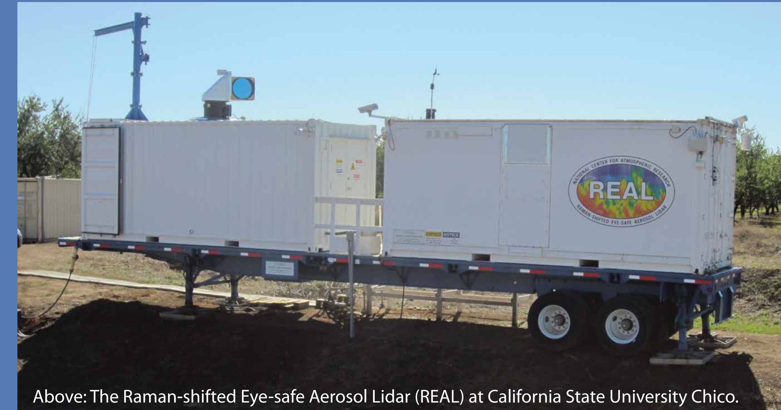
Above: The Raman-shifted Eye-safe Aerosol Lidar (REAL) at California State University Chico.
