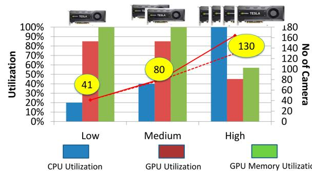
\*\*Based on the fixed frame rate of 15fps and Dual 8 core CPU, different system configurations indicating the scalability of the number of camera per system however, increment of GPU cards to scalability factor is non-linear due CPU capability.
