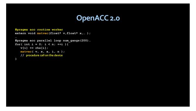
Here, the routine directive appears just above the prototype for the procedure. This tells the compiler that there will be a device copy of the routine 'matvec.' It also tells the compiler that there may be a loop in 'matvec' that targets the worker-level parallelism, so calls to 'matvec' may not appear within a worker loop. Essentially, it says that worker-level parallelism has to be reserved to the routine 'matvec,' and may not be used by the caller.
