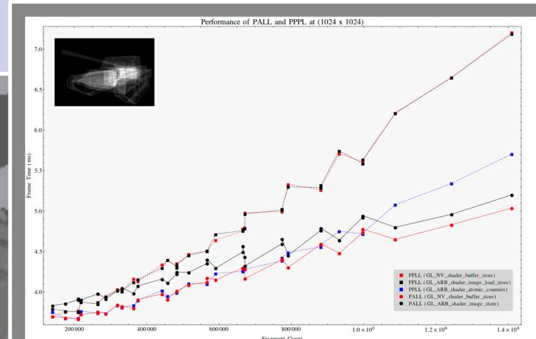
The performance of PALL and PPLL on an NVIDIA GeForce GTX 690 using OpenGL 4.3. When PALL and PPLL use the same counters, PALL is consistently faster than PPLL. Furthermore, PALL performance is on par with PPLL when PPLL uses the fastest atomic counters. Unfortunately, PALL cannot use the fastest atomic counters as they do not provide atomic add operations, only atomic increment.
