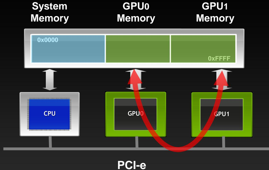
**Direct Transfer & Direct Access between GPUs**
