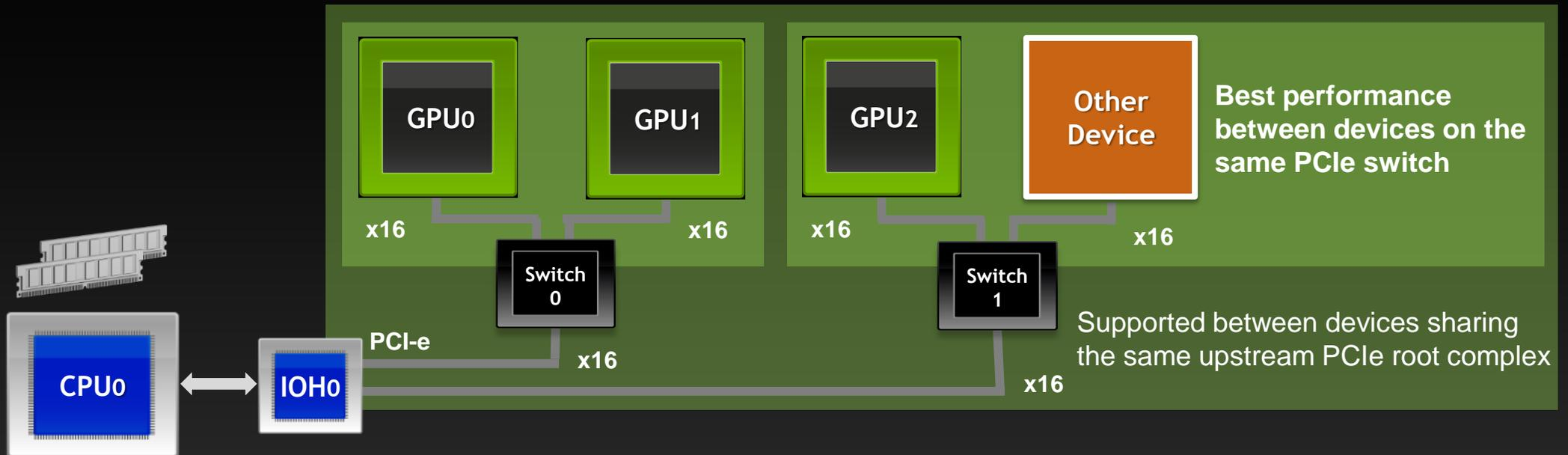
PCI-e Switches: **Fully Supported**
